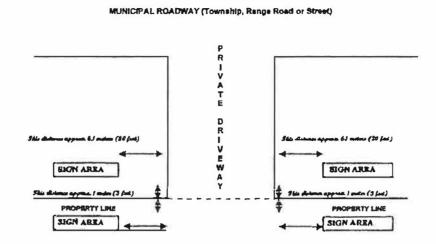
Signs shall be placed within 6.1 meters (20 feet) on either side of the shoulder of the driveway (approach) and located 1 meter (3.3 feet from the property boundary either within the property boundary or within the road right-of-way boundary. The sign shall be no tower than 1 meter (3.3 feet) from ground level (measured from bottom of sign) and no higher than 2 meters (6.6 feet) from ground level (measured from top of sign).
