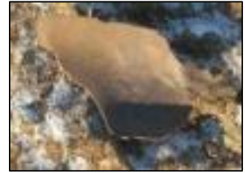
Metal fragment from the fatal 2016 propane cylinder explosion.
