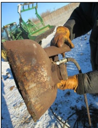
Photograph from the 2016 fatality investigation showing the top of the ruptured propane cylinder.
